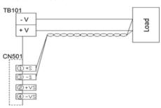
If no Remote Sensing will be used, please retain CN501 jumper connector as shown:
